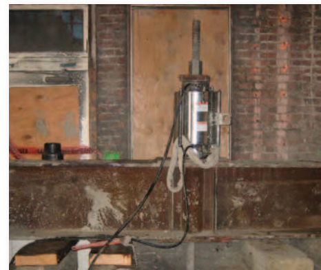
Figure 13: Tension testing apparatus
